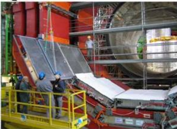
Housing containing 6 HO modules being installed in CMS detector
