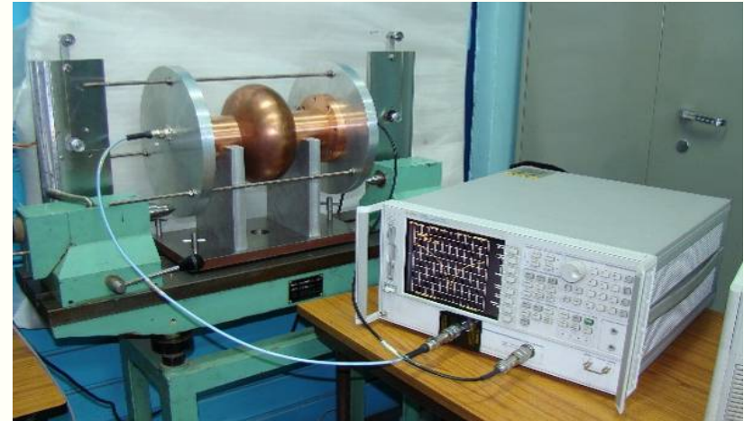
Bead Pull Measurement Setup for Assembled Cavity
